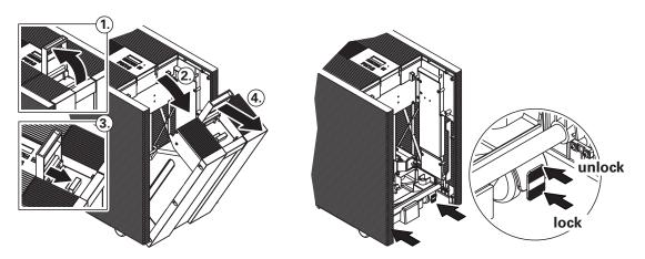
• Completely unwind the mains cable (at the point of the delivery the mains cable is winded up in the unit) and take it out of the unit as shown below.
